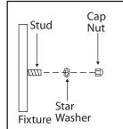
Install the light fixture to the wall by aligning the hole(s) in the fixture with the studs on the mounting bracket. Secure in place with cap nut(s) and star washer (s).
