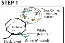
Attach easy connect mounting bracket to electrical box with electrical box screws (not included).
