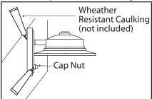
After Installation, seal around the top and side perimeter between the fixture and the wall surface with weather resistant caulking. The bottom should be left un-caulked to prevent moisture build-up. Apply a small amount of weather resistant caulking around the side perimeter between the cap nut and mounting plate.
